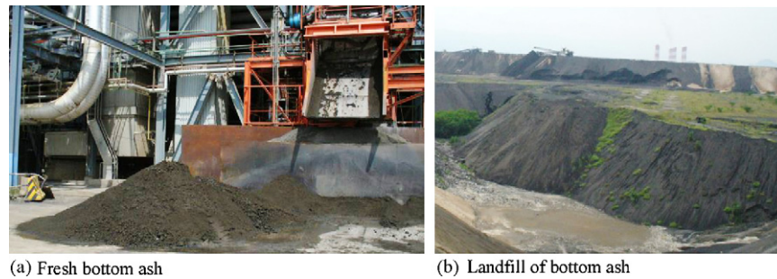
Fig. 1. Fresh bottom ash and landfill of bottom ash at Mae Moh power plant. (a) Fresh bottom ash and (b) landfill of bottom ash.
